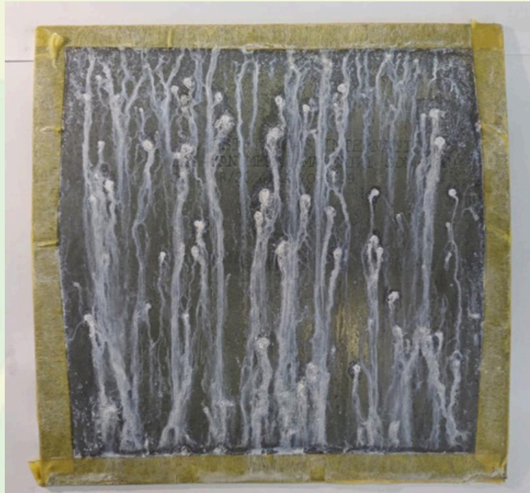
Photo 1.2: Metal plate after NSS 1000hrs (Front view).
